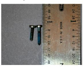
NOTE: Screw torque should be set at 16 Ncm +/-2 Ncm. This can only be achieved with a properly calibrated torque driver. All torque drivers should have routine inspections for correct calibration and proper performance.
